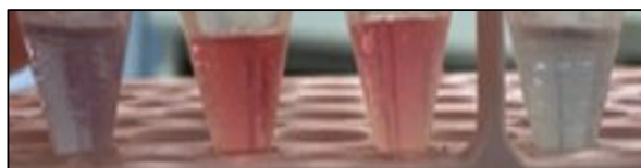
Figure 3.8 The color of EDC/NHS-AuNPs@SER at pH from left to right 2.3, 5.4, 7.4 and 10.0, respectively
