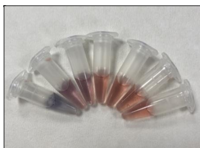
Figure 3.13 The color change of EDC/NHS-AuNPs@SER probes in 5 to 500 \mu\text{M} of Neu5Gc standard solutions, respectively
