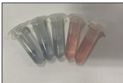
Figure 3.16 The color of DSP-AuNPs@SER at pH from left to right 2.0, 3.0, 4.0, 9.0, and 11.0, respectively
