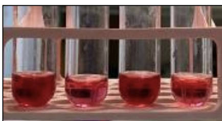
Figure 3.9 The color of EDC/NHS-AuNPs@SER solutions at pH from left to right 5.4 in the absence of Neu5Ac, at pH 5.4 in the presence of Neu5Ac, at pH 7.4 in the absence of Neu5Ac, at pH 7.4 in the presence of Neu5Ac, respectively. Reaction time was 5 min
